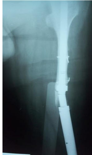
picture 2 X-ray of the thigh bone of a boy of 16 years: a fracture of the foot of a cementless endoprosthesis
